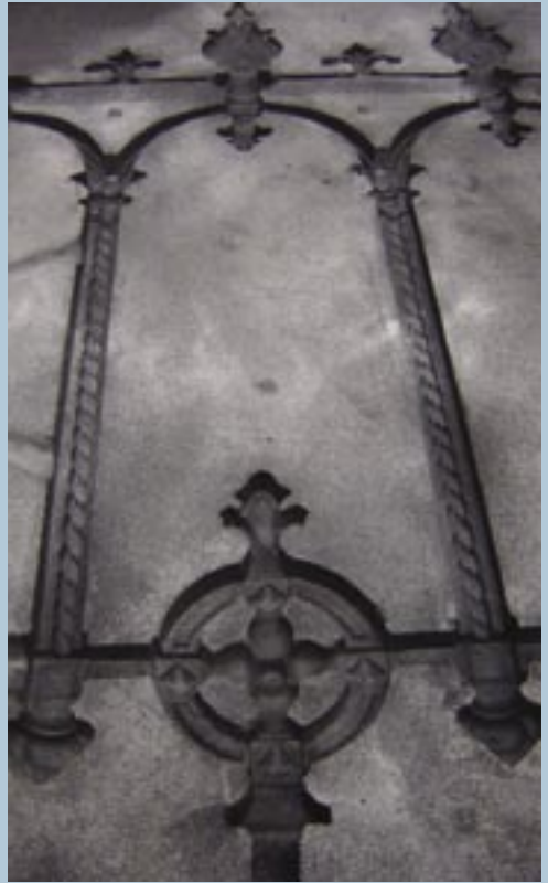
Image: Open greensand mould for baluster panel.
